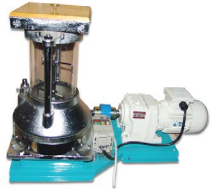
VİTAMİN MAKİNASI Vitamin ( Micro Ingradient Feeding Unit )
